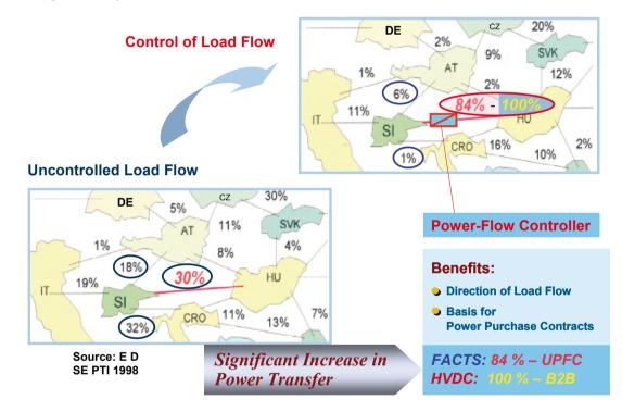
Fig. 34 a): Load-Flow Improvement with Power-Flow Controller
