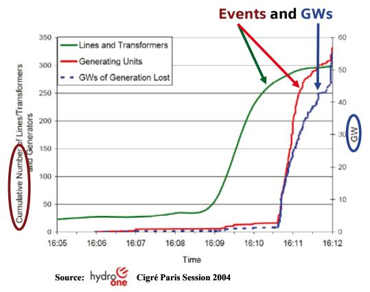
Fig. 14: Recordings from HydroOne – from 16:05 to 16:12
