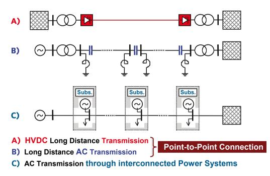
Fig. 26: Network Configurations for Long Distance Transmission
