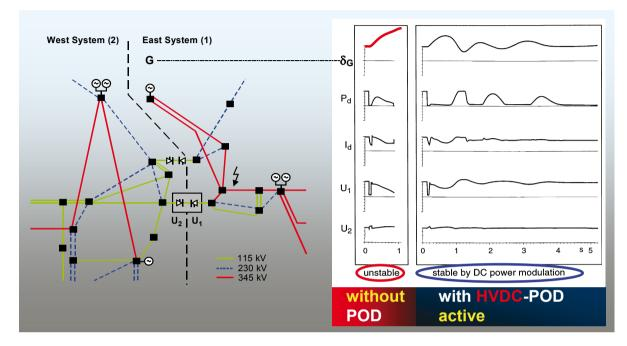
Fig. 31: Interconnection of Separated Grids in USA, Voltage Control and Damping of Power Oscillations - HVDC B2B - Virginia Smith Converter Station
