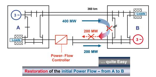
Fig. 34 b): Elimination of Loop Flows by means of Power-Flow Controller
