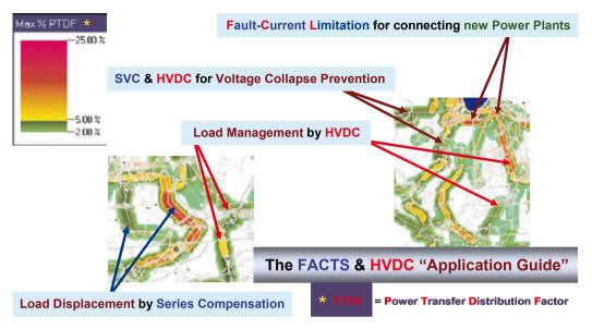
Fig. 27: Elimination of Bottlenecks in Transmission - Prevention of Overloads and Outages
